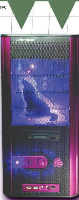
The howling wolf that graces the front uses two LEDs. "I actually cut the wolf out of acrylic, sanded both sides with 160-grit paper to make it foggy and opaque, and then I reduced the image size by about 20 to 30% and printed off a template for the 'blacked-out wolf' and cut that out of poster board and sprayed that black with vinyl-dye paint," says Tate.
